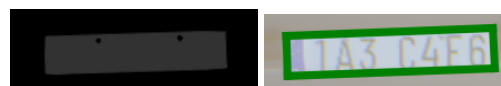
Figure 8: Semantic segmentation by BERGE simulator and bounding box detection by Unicam LP detection.
